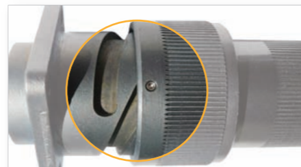
Legendary Cannon bayonet coupling design allows for fast and easy mating and unmating. An audible sound and visual indication, realized by a color marked snap-in position indicator, offer additional coupling security and vibration resistance up to 20 g's.
