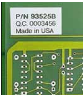
Circuit board labeling
