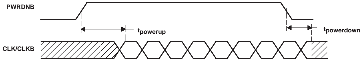
Figure 8. PWRDNB Transition Timings
