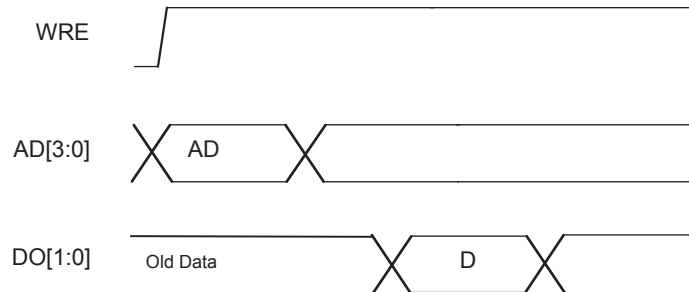
Figure 3-7. Slice Single /Dual Port Read Cycle Timing
