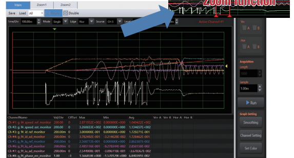
Display variables for 8 channels (can specify scale and off-set settings etc. per channel)
