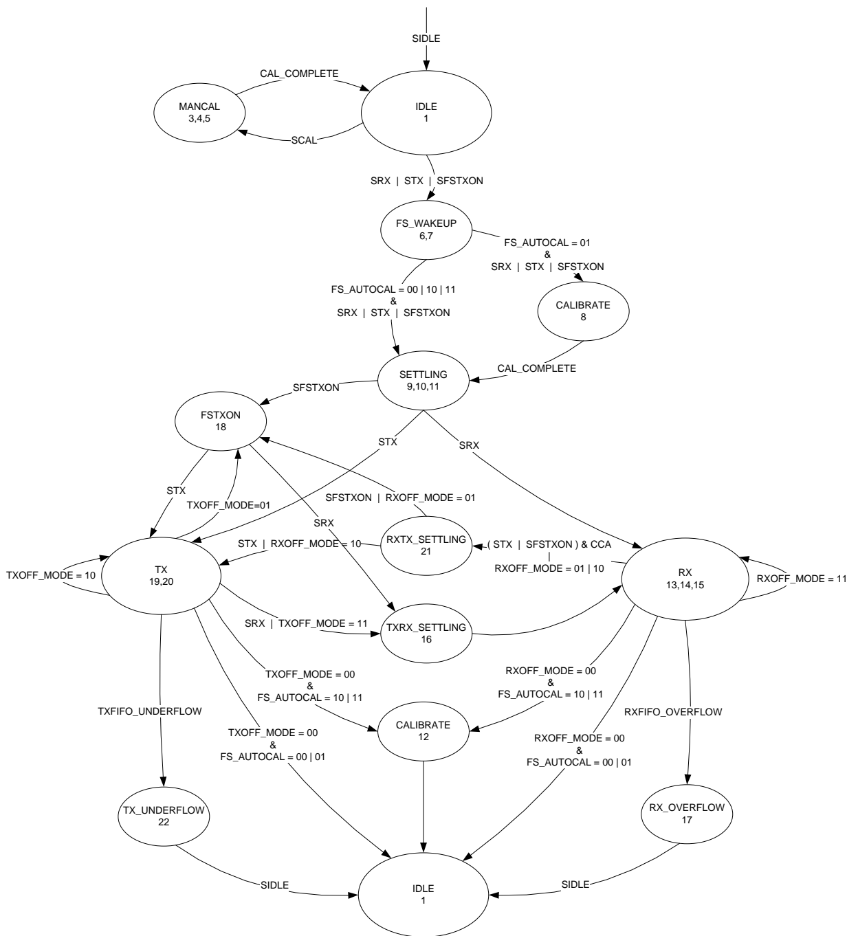
Figure 54: Complete Radio Control State Diagram
