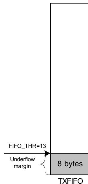
Figure 5-14. Example of FIFO at Threshold
