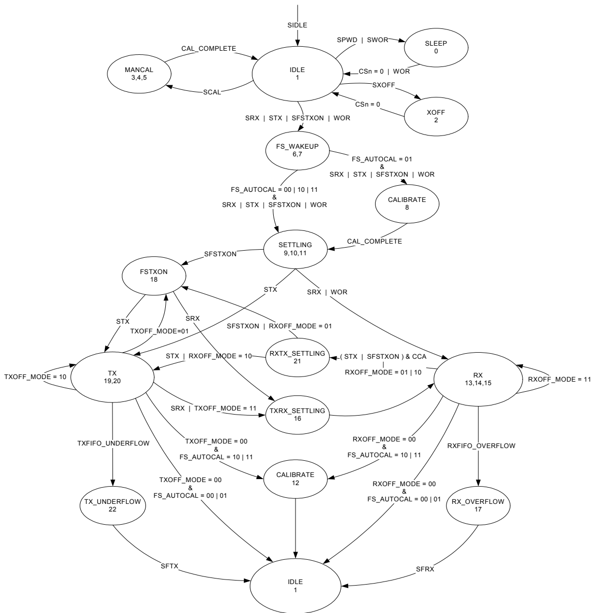
Figure 16: Complete Radio Control State Diagram
