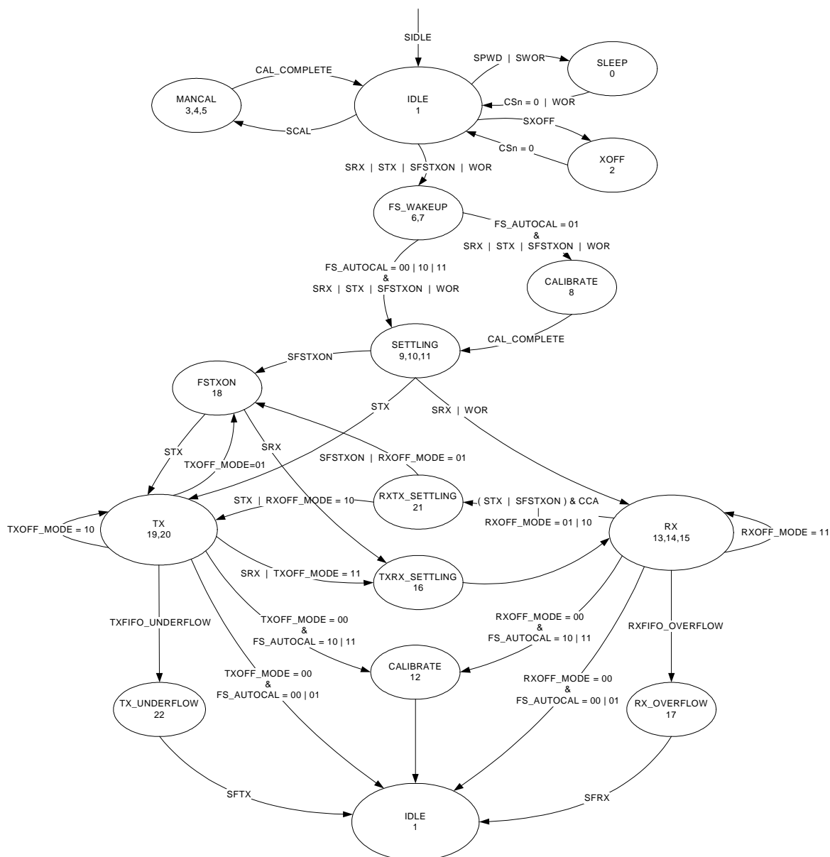
Figure 20: Complete Radio Control State Diagram
