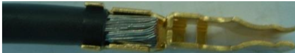
Picture 4. Wire and Terminal before Crimping
