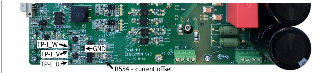
Figure 4 Relevant parts for offset adjustments
