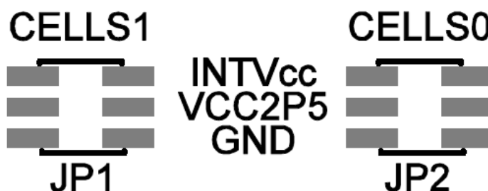
Figure 2. Cell Count Configuration Jumpers
