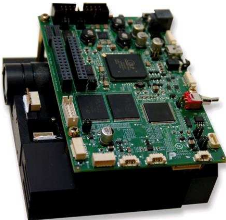
Figure 1. DLP LightCrafter 4500 Evaluation Module (EVM)
