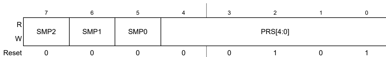
Figure 16-7. ATD Control Register 4 (ATDCTL4)
