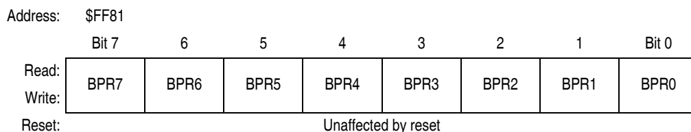
Figure 2-8. FLASH-2 Block Protect Register (FL2BPR)
