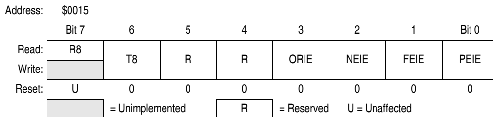
Figure 13-12. ESCI Control Register 3 (SCC3)
