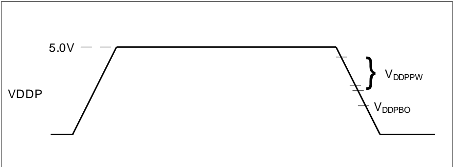
Figure 12 Supply Threshold Parameters
