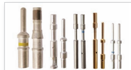
The CA Bayonet contacts incorporate copper alloy plated with a hard silver finish (optional gold) and guarantee at least 500 mating cycles. All solder contacts feature a special passivation to comply with RoHS requirements.
