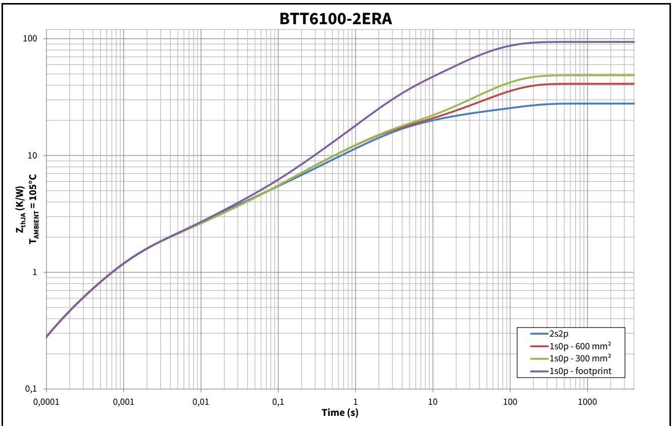
Figure 6 Typical Thermal Impedance. 2s2p PCB set-up according Figure 5
