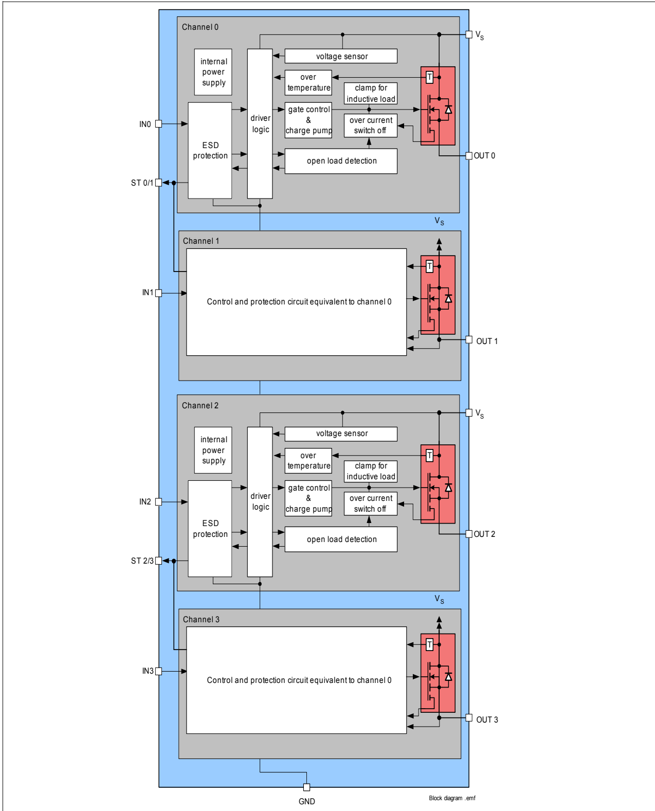
Figure 1 Block diagram for the BTS4130QGA
