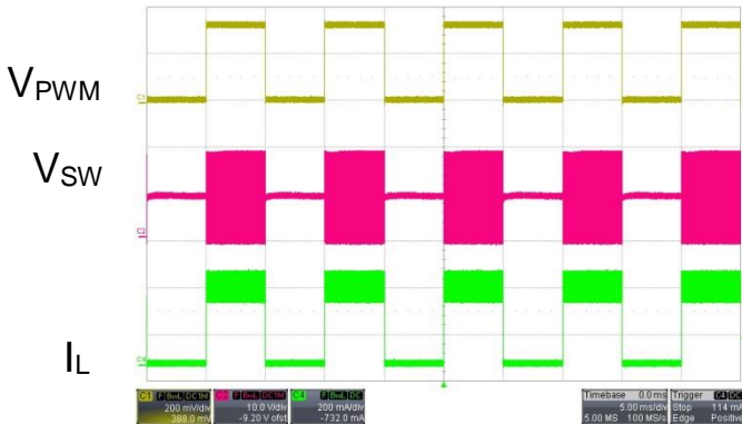
R_S Short ( V_{LED}=9\text{V} , R_S=0.3\Omega , L=47\mu\text{H} )
