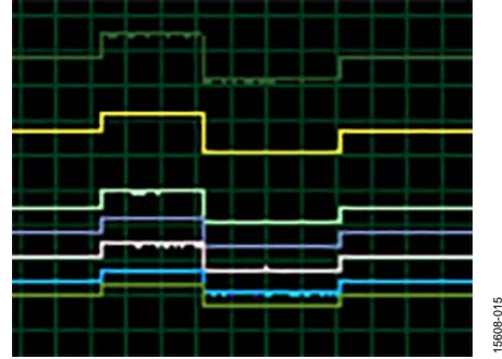
Figure 15. Rails Going from Nominal Setpoint to Margin High, Margin Low, and Back to Nominal Voltage
