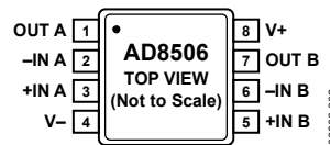
Figure 3. 8-Lead MSOP (RM-8)
