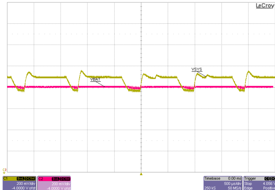
Figure 16. V(SYS) when Reverse Boost Prevention Circuit is Active
