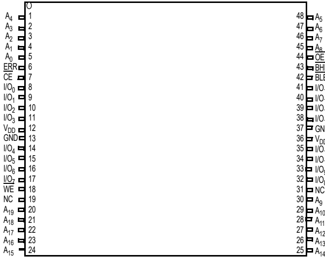
Figure 7. 48-pin TSOP I (12 × 18.4 × 1 mm) Pinout, Single Chip Enable with ERR, CY7C1061GE [7, 8] Package/Grade ID: ZXI
