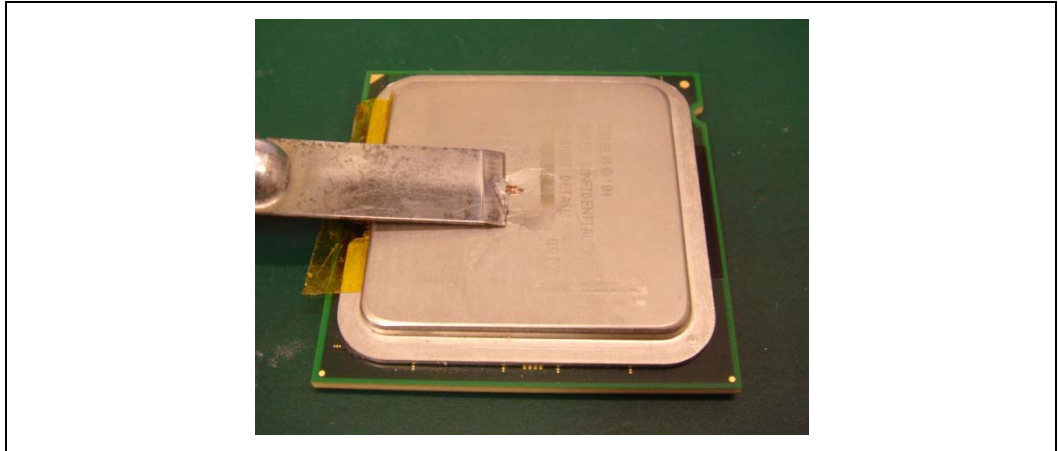
Figure 7-35. Removing Excess Adhesive from IHS
