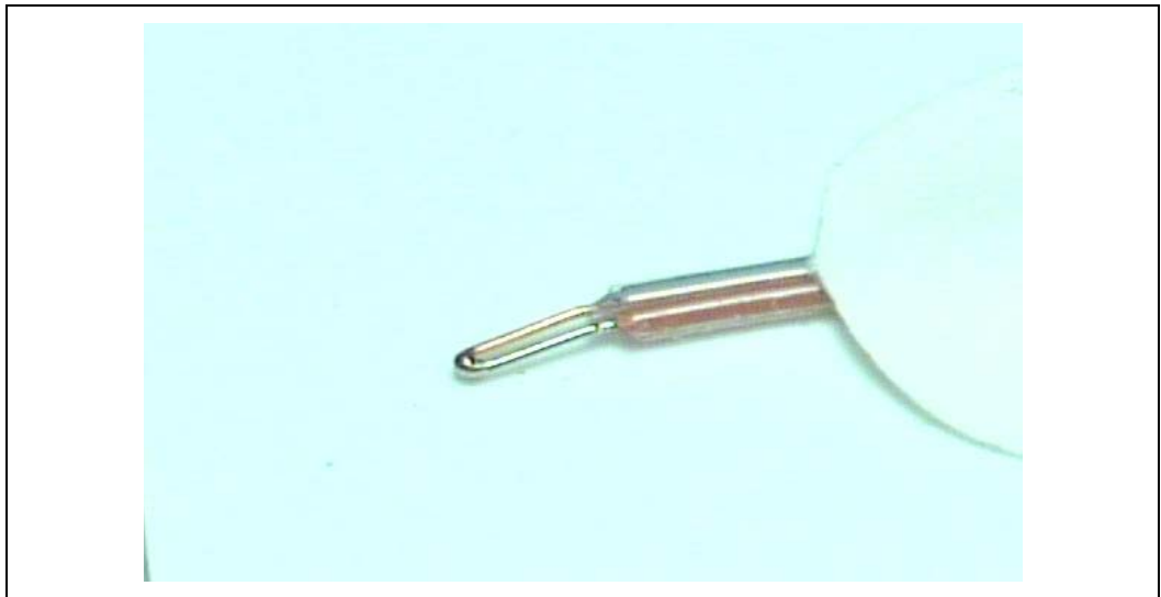
Figure 7-16. Inspection of Insulation on Thermocouple
