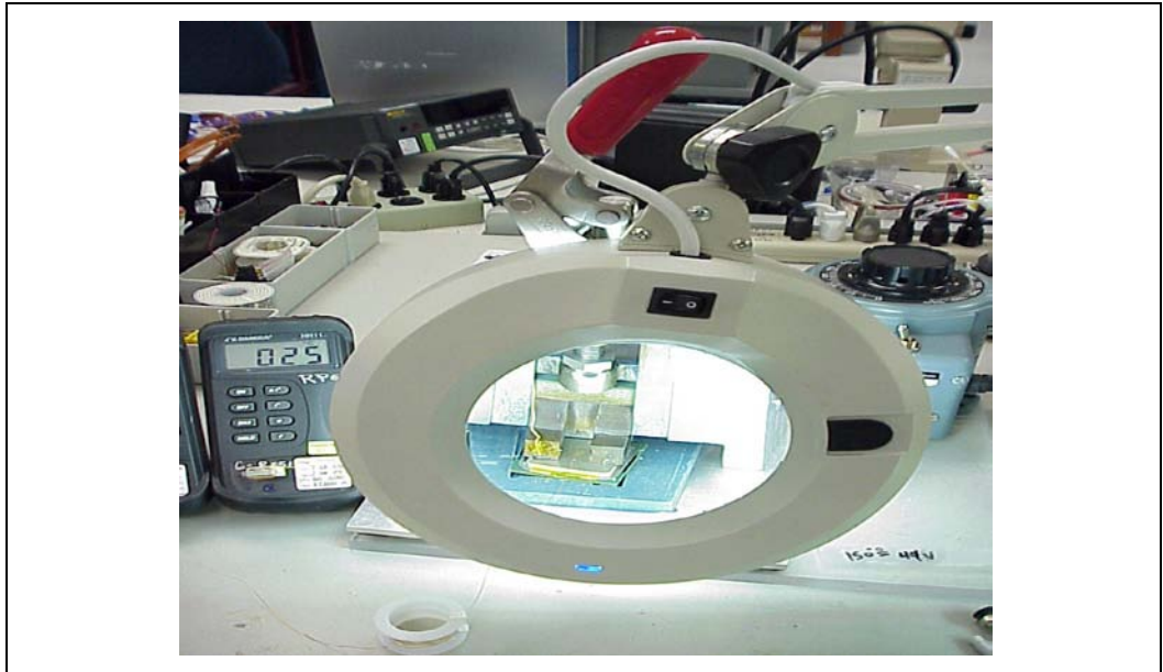
Figure 7-29. Moving Solder back onto Thermocouple Bead
