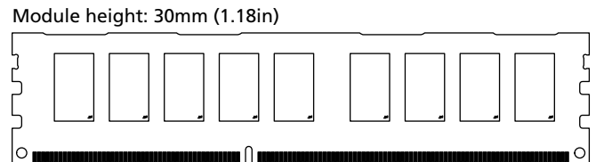
Figure 1: 240-Pin UDIMM (MO-269 R/C E)
