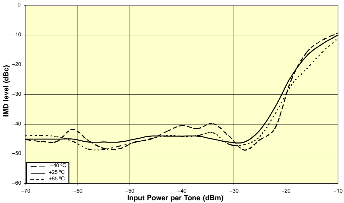
Figure 5. IMD Level vs Temperature at Output AGC Setting of 1.2-Vpp Differential (IF2 Filter Loss of 15 dB Included)
