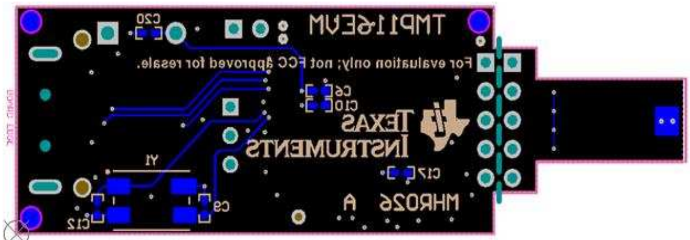
Figure 26. Bottom Assembly Layer
