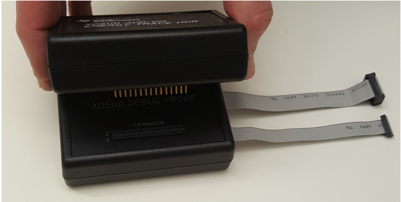
Figure 4. The XDS110 Probe and ETHDR System
