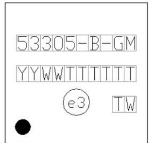
Figure 8.6. Si53305 Top Marking
