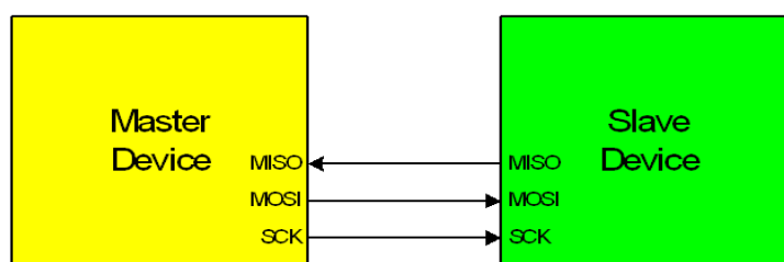
Figure 30.3. 3-Wire Single Master and Slave Mode Connection Diagram
