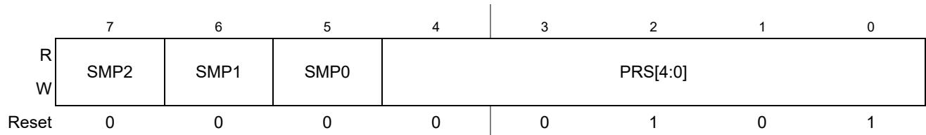
Figure 14-7. ATD Control Register 4 (ATDCTL4)
