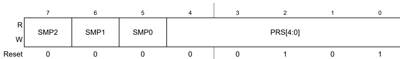
Figure 13-7. ATD Control Register 4 (ATDCTL4)
