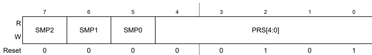
Figure 15-7. ATD Control Register 4 (ATDCTL4)
