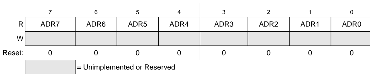
Figure 9-6. Data Result Low Register (ADCRL)
