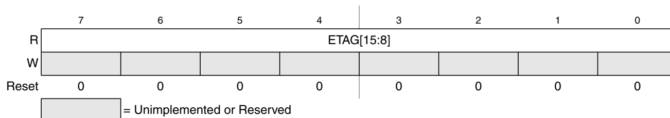
Figure 25-18. EEE Tag Counter High Register (ETAGHI)
