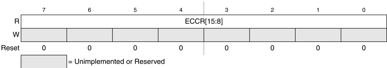
Figure 28-20. Flash ECC Error Results High Register (FECCRHI)
