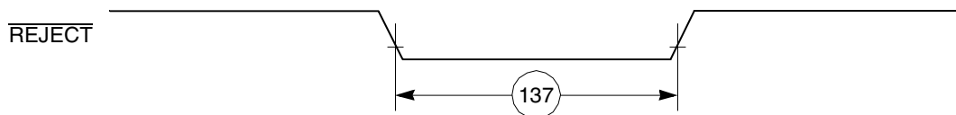
Figure 58. CAM Interface \overline{\text{REJECT}} Timing Diagram
