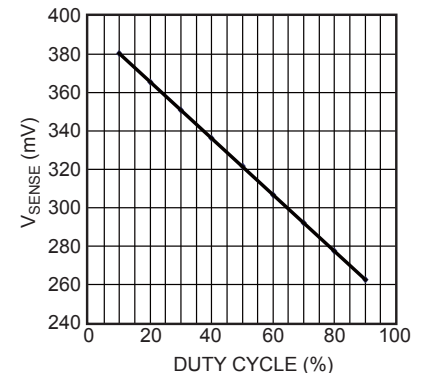
Figure 2: V SENSE vs Duty Cycle
