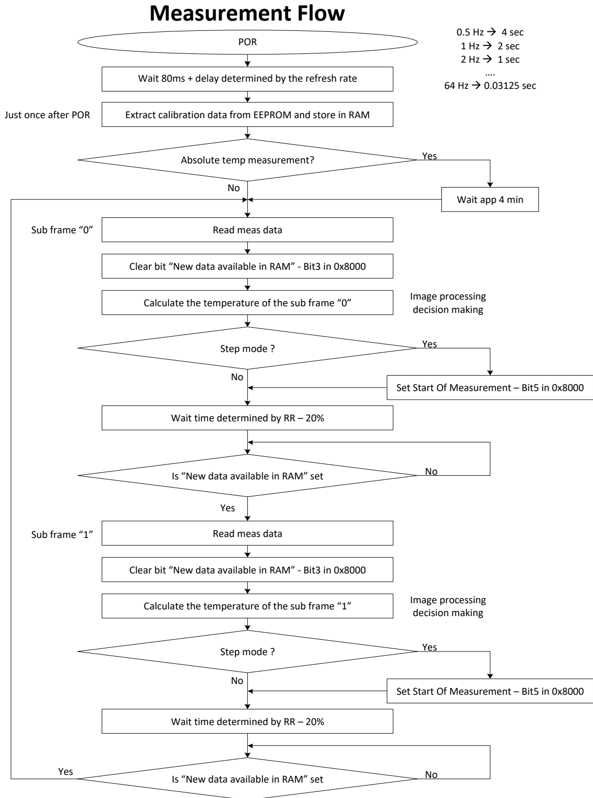
Figure 7 Recommended measurement flow
