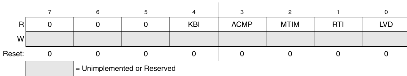
Figure 5-7. System Interrupt Pending Register (SIP1)
