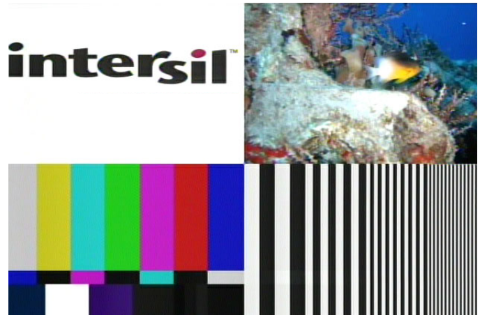
FIGURE 18. TEST PATTERN IMAGE AFTER 5200 FEET OF CAT 5 WITH ISL59605
