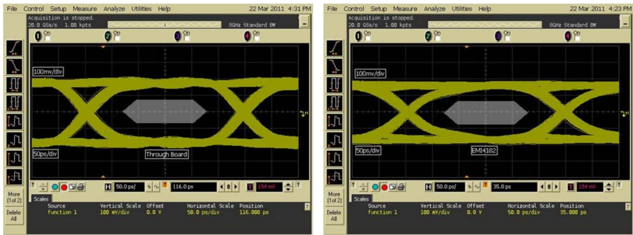
Figure 10. EMI4162MU Measured Eye Diagram @ 3.4Gbps (EVB through on left, EVB with EMI4162 on right)
