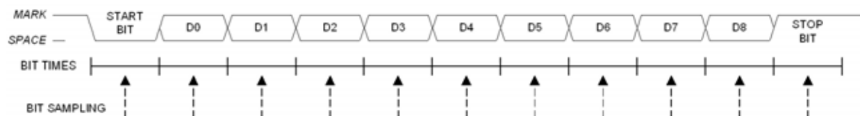
Figure 25.5. 9-Bit UART Timing Diagram
