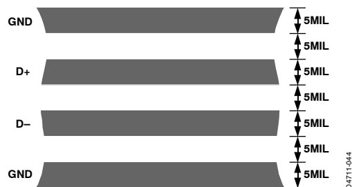
Figure 25. Arrangement of Signal Tracks
