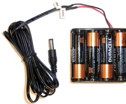
Figure 49. Recommended Power Supply for ADS1x98ECG-FE
