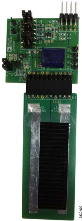
Figure 2. ADP5090-2-EVALZ Board Hardware
