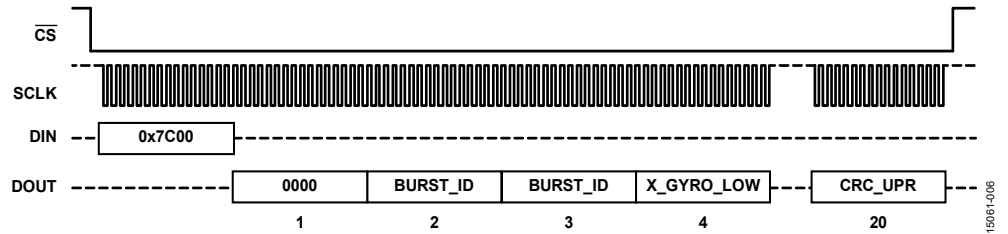
Figure 6. Burst Read Function Sequence Diagram, 20 Segments
