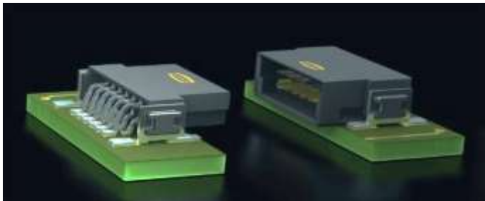
Extender Card (2 angled connectors)
