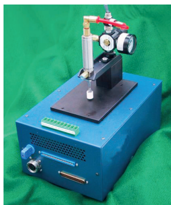
Figure 3-9: \theta_{JC} Measurement Setup
