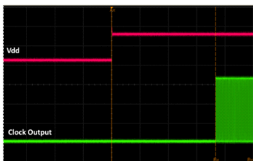
Figure 17. Startup Waveform vs. Vdd
