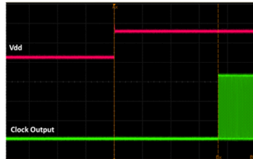
Figure 17. Startup Waveform vs. Vdd
